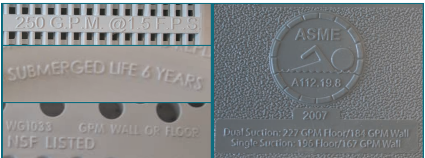
Photo 5: Examples of compliant drain cover markings.
